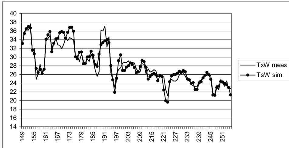
Figure 6 Measured and simulated minimum water temperatures. Opera, 2002
