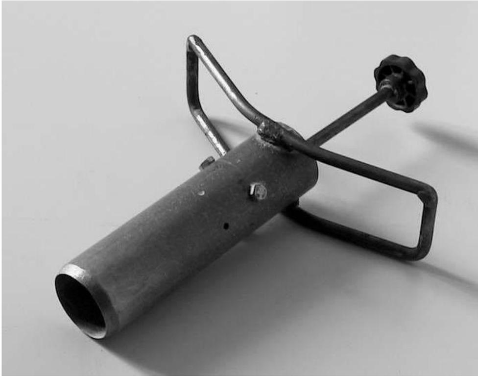
Figure 1. Prototype of the soil sampler for paddy fields
