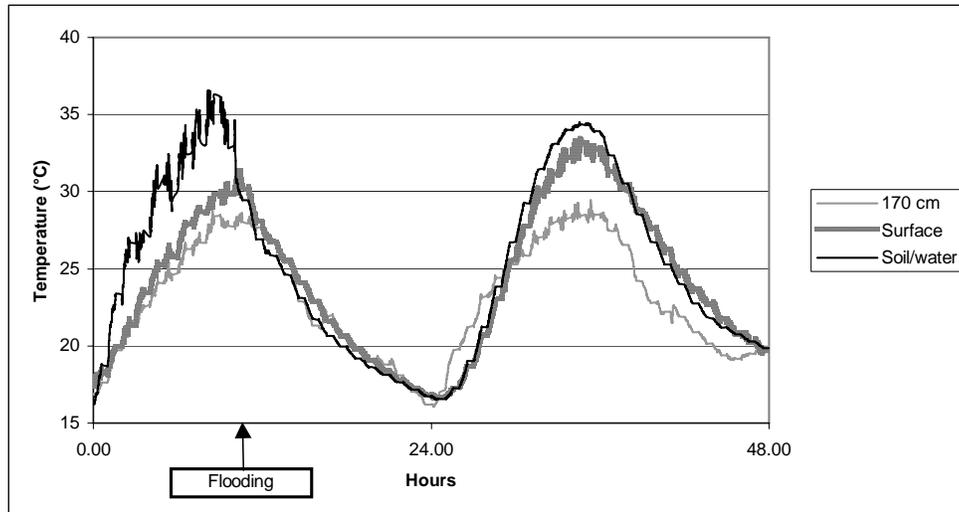
Figure 3 – Temperature measured at different levels with the floating station (Vignate (MI); 48 hours starting from June 1 2002; 6.00 am) at the soil/water interface, on the surface and at 150 cm from water surface. The flooding effect on water temperature is evident in the second day, when water produces a significant delay in the afternoon temperature decrease
