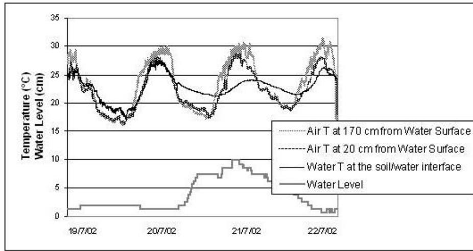
Figure 1 Water level measurements and hourly temperatures gauged at soil/water interface (water temperature), at 20 cm and at 170 cm from water surface (air temperature). Data from rice field of Vignate
