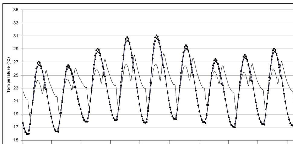
Figure 4 Hourly temperatures for air (line with triangles), for canopy layer 70-80 cm (line with dots) and for water surface (normal line) simulated by the mechanistic model (station of Vignate / period 25 July – 4 August 2002)
