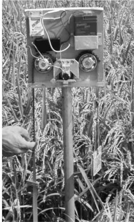
Figure 1. The water level sensor (with opened case)
